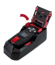
2. Keeping the charge clips connected, lie G7 down into dock and push down until it clicks in place.
